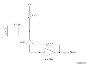
For the MPPC readout circuit, a current-to-voltage amplifier can be used as with previous semiconductor devices. The MPPC outputs high-speed pulse signals, but because the gain of the MPPC itself is high, there is no need to greatly increase the gain on the circuit side. This has an advantage that there is more freedom in circuit design.
