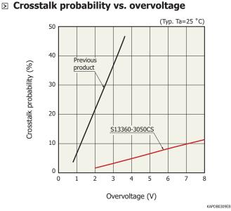
Note: Dark pulse overlap (pile-up effect) is eliminated.
